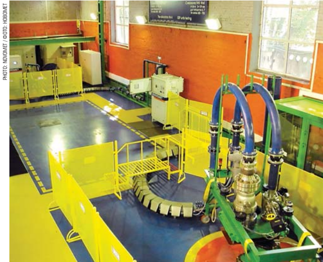
ESP testing laboratory at BN KONNAS experimental design bureau (Moscow).
